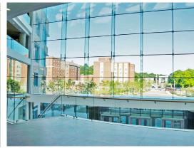
Track Rail glass stair and segmented overlook railings are mechanically fastened to structural steel finished off with aluminum cover plates.
