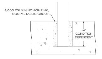
Notes: Handrails can be mounted to concrete or steel. Anchor size/Type may vary due to field conditions.
